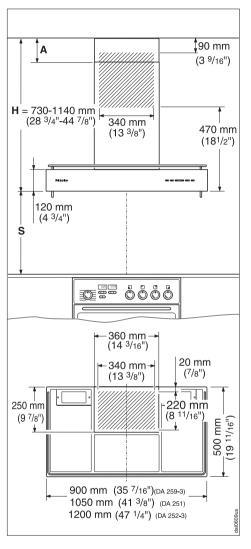
Cut out area in wall or ceiling for entrance of 6" (150 mm) ductwork or 5" (125 mm) ductwork with a reducing collar.
